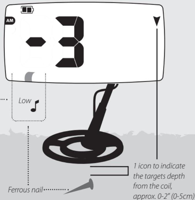
Metal detectors work due to the fact that metal is conductive. Metal detectors create an electromagnetic field, which penetrates the ground.
